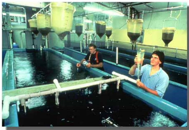
Water quality in the 7,400-gallon recycled-water system must be monitored closely. Here, culture assistant Eric Leonard (right) and system manager Joe Hankins check levels of acidity and solids. (Photo by Scott Bauer, USDA-ARS)
